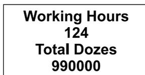
**Working Hours** represents the total Nr. of hours that motor run since fabrication
